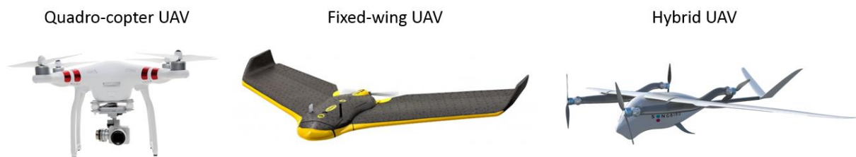
Figure 2: Example UAV platforms - Phantom 3 (DJI), Ebee (SenseFly), Songbird (Aerolution)
