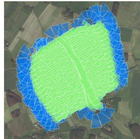
Figure 1: Flight pattern, green images are selected for photogrammetric processing
