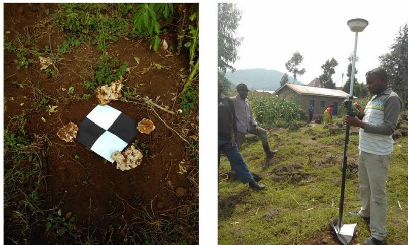
Figure 2: Measurement of ground reference points
