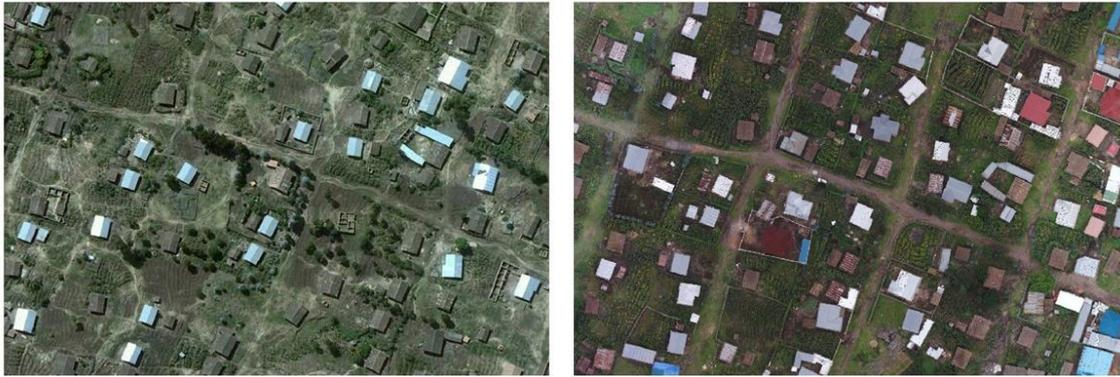
Figure 4: Left: Orthomosaic based on aerial images from 2009; right: Orthomosaic based on UAV images from 2018
